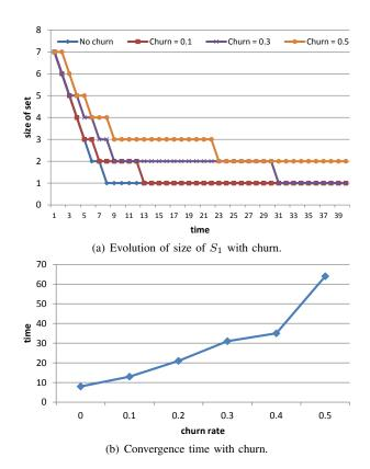
Fig. 8. Impact of churn with  $T_C = 0.97$ . As expected, high churn delays convergence since the system has less chance to learn and adjust the reputation of nodes.
