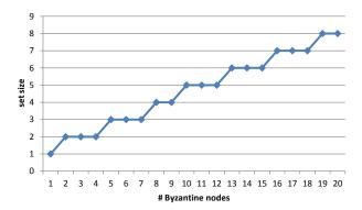
Fig. 6. Size of  $S_1$  for  $T_C = 0.97$  when b varies. When the system is stable, the adding of several Byzantine nodes increases the number of nodes needed to be contacted.
