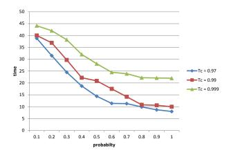
Fig. 5. Convergence time to reach the minimum size of S1 (|S1| = 1) when the probability of the Byzantine node to return a wrong value varies. A smart Byzantine node with sporadic wrong value computation highly increases the convergence time.
