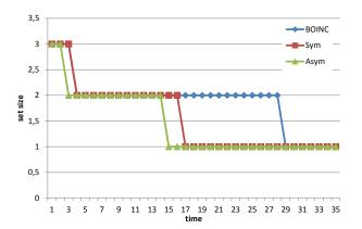
Fig. 4. Evolution of size of S1 for b =1 and  $T_C = 0.97$  for the 3 reputation strategies. By keeping the highest difference between the reputation of correct and Byzantine nodes, the asymmetric strategy quicker converges to the smallest value of S1.
