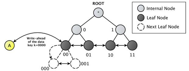
**Fig. 4:** Write-ahead protocol example: insertion of data key  $k=0000$ .
