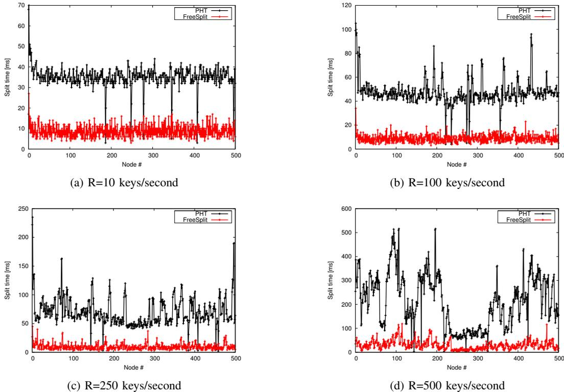
Fig. 6: Split time when indexing an uniform distribution for different insertion rates
