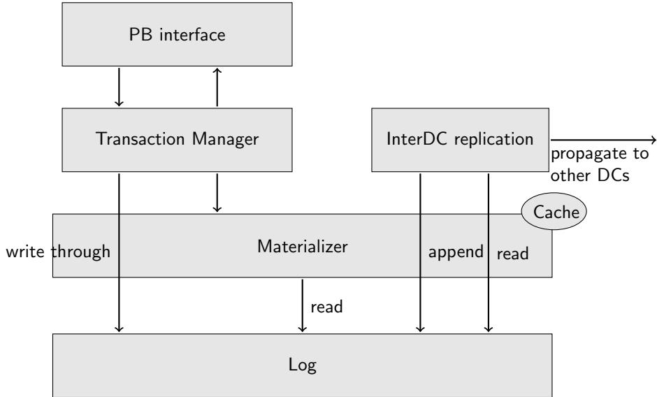
Figure 1: Architecture of Antidote.
